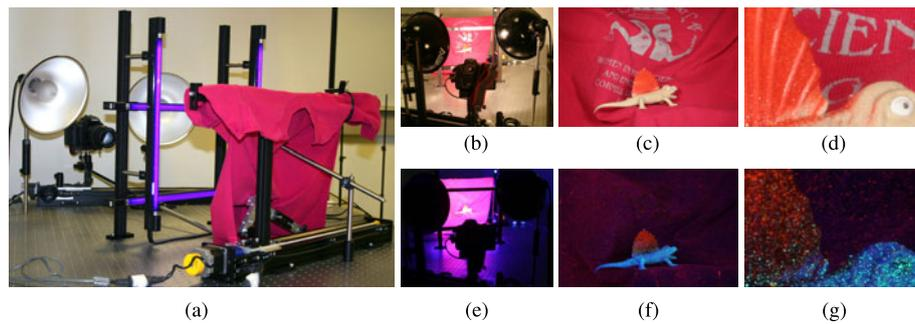
**Fig. 1** (a) The setup for obtaining ground-truth flow using hidden fluorescent texture includes computer-controlled lighting to switch between the UV and visible lights. It also contains motion stages for both the camera and the scene. (b–d) The setup under the visible illumination. (e–g) The setup under the UV illumination. (c and f) Show the
